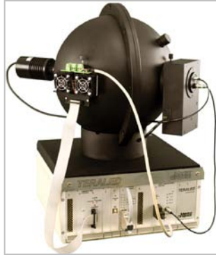
A Ø30cm sphere with a Ø60mm DUT LED port for LEDs up to 10W with a filter based detector system.
