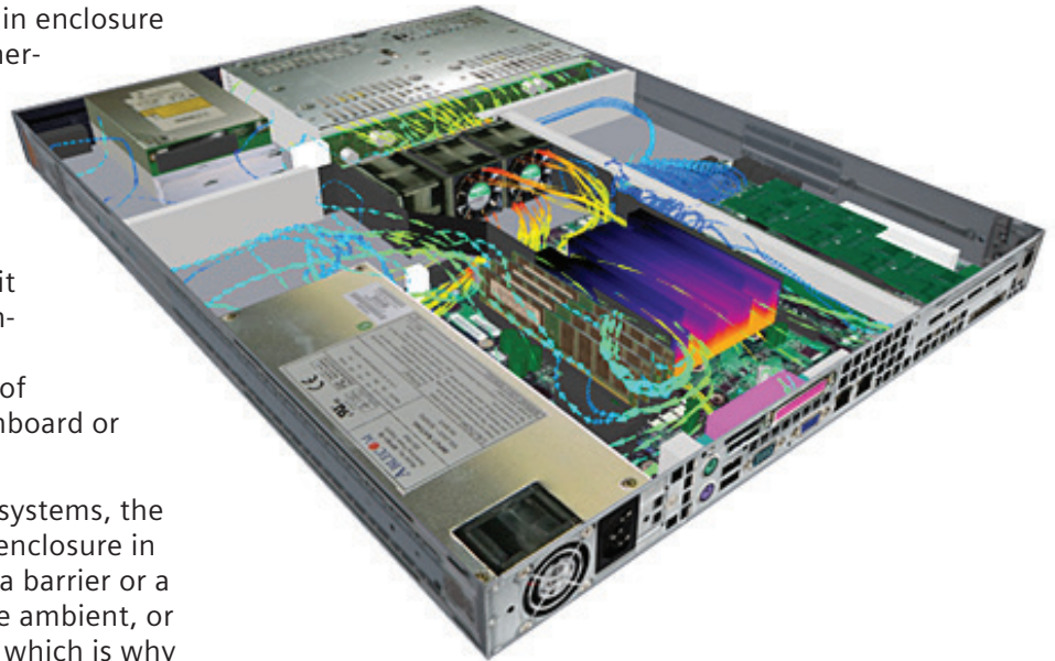
Figure 1: Airflow distribution in a 1U server modelled in Simcenter Flotherm
